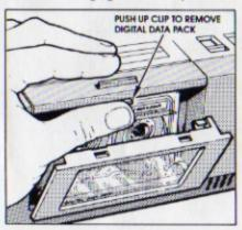
The easiest way to insert a data pack is to lay the data pack against the drive door. Make sure the data pack is centered, the label is facing out, and side of the data pack where the tape shows is down. Then close the door by pushing on both sides of the door simultaneously.
