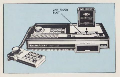
When removing the GAME CARTRIDGE, simply pull it straight up and out of the slot. **Remember to turn the POWER SWITCH** "**OFF**" when removing the CAR-TRIDGE. The POWER SWITCH on ColecoVision<sup>™</sup> CONSOLE should be turned "OFF" when game is not being used.
