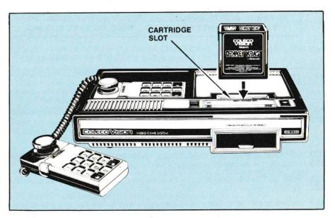
When removing the GAME CARTRIDGE, simply pull it straight up and out of the slot. Remember to turn the POWER SWITCH "OFF" when removing the CARTRIDGE. The POWER SWITCH on ColecoVision™ CONSOLE should be turned "OFF" when game is not being used.
