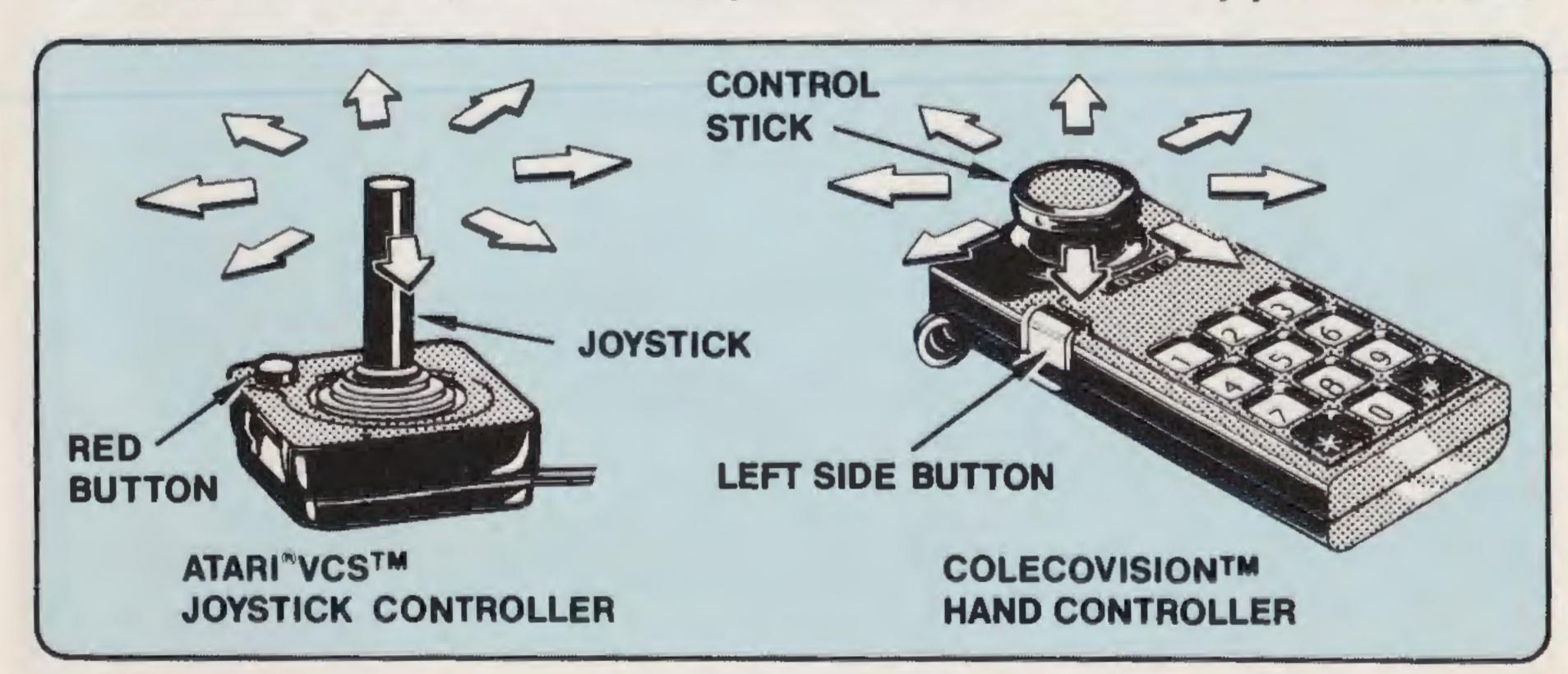
The **left** side button on your standard ColecoVision™ hand controller functions just like the red button on the Atari® VCS™ joystick controller.
