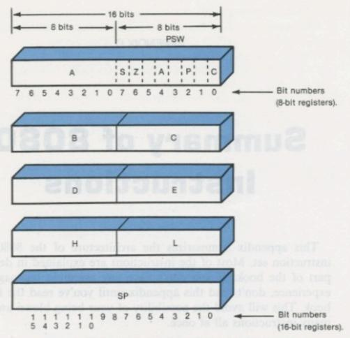
Fig. C-1. Registers of the 8080 microprocessor.
