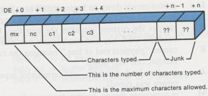
Fig. 3-2. Buffer address in the DE register.
