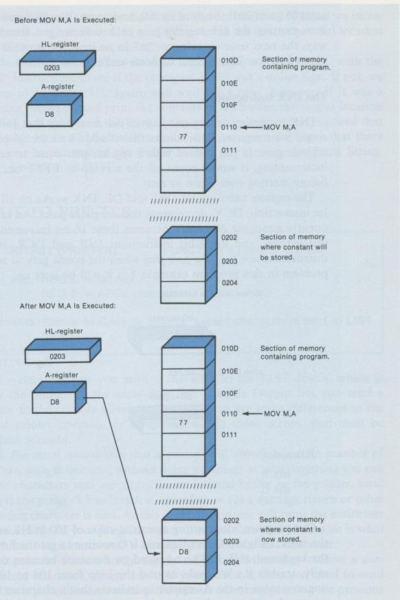
Fig. 3-6. The phantom "M" register.
