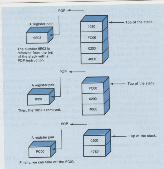
Fig. 2-8. Using the POP to manipulate the stack.
