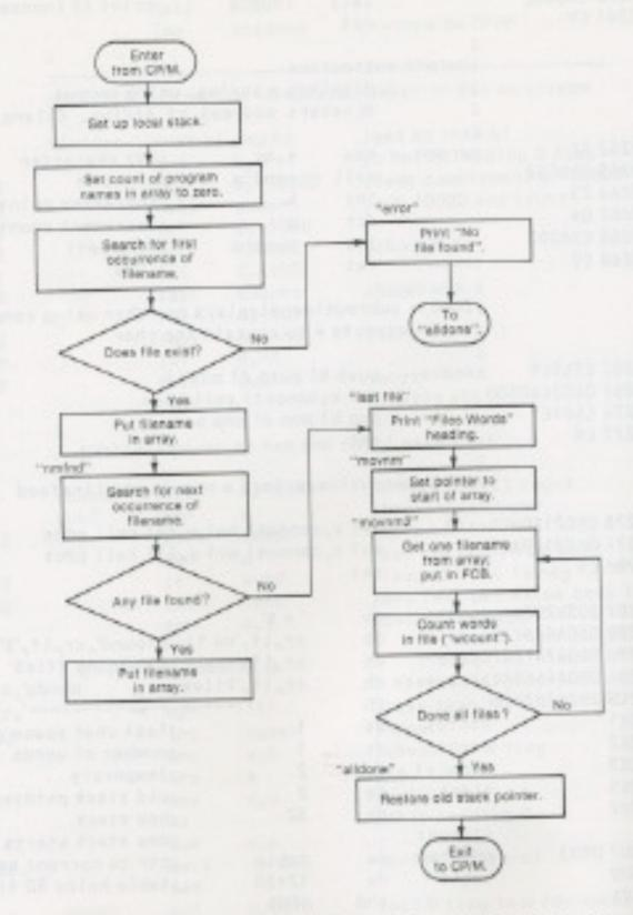
Fig. 7-4. Flowchart of the "WORDS" portion of the program in Listing 7-1.
