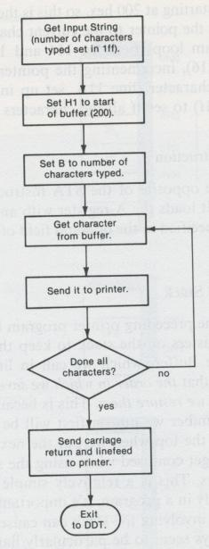
Fig. 3-8. Flowchart for outputting data to the printer.
