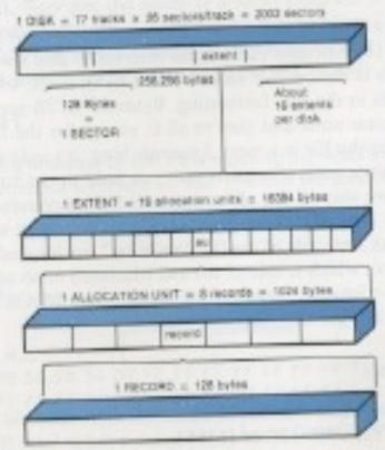
Fig. 7-3. The relationship of records, allocation units, sectors, etc.
