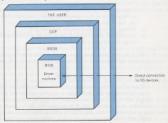
Fig. 9-1. BIOS communicates with I/O devices.
