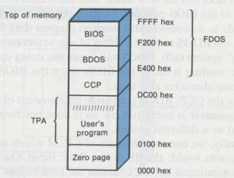
Fig. 1-2. The parts of CP/M.
