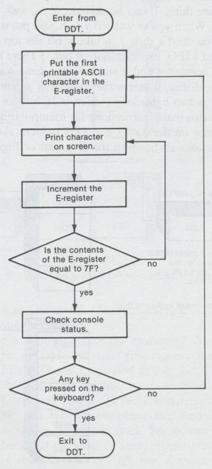
Fig. 2-6. Flowchart of the Barber-Pole Display program.
