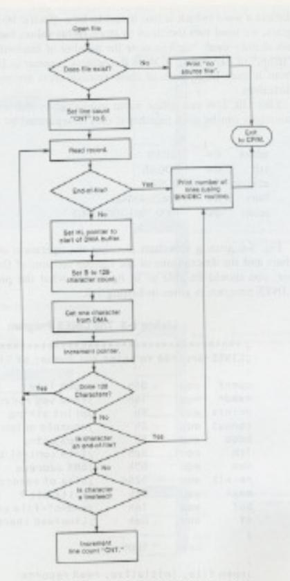
Fig. 5-6. Flowchart for the LINES program.
