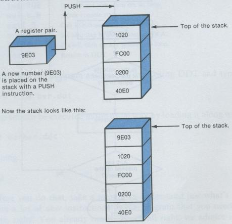
Fig. 2-7. Using the PUSH to manipulate the stack.
