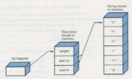
Fig. 8-6. Using a three-byte descripter.
