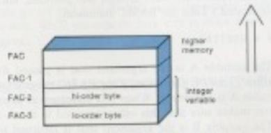
Fig. 8-5. The Floating Pointer Accumulator.
