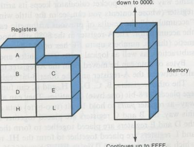
Fig. 1-7. The principal parts of the 8080 microprocessor.
