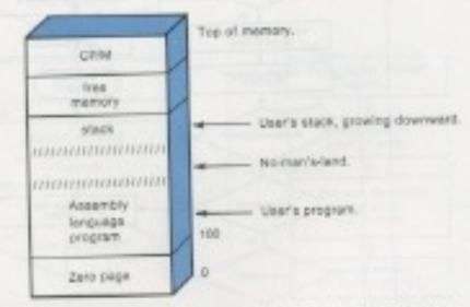
Fig. 7-6. Location of the user's program and the stack.
