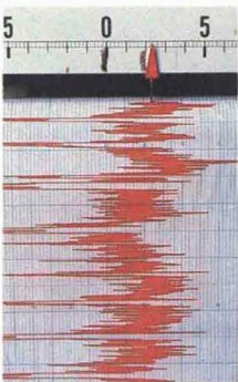
Scanner monitors thickness of extruded vinyl.
