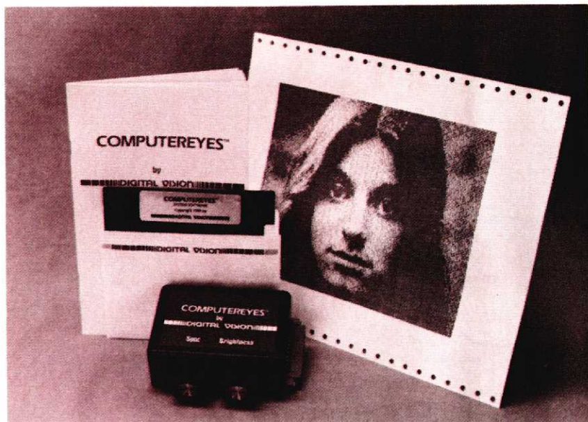
Computereyes lets you digitize images using a Commodore 64 or Apple II series computer.
