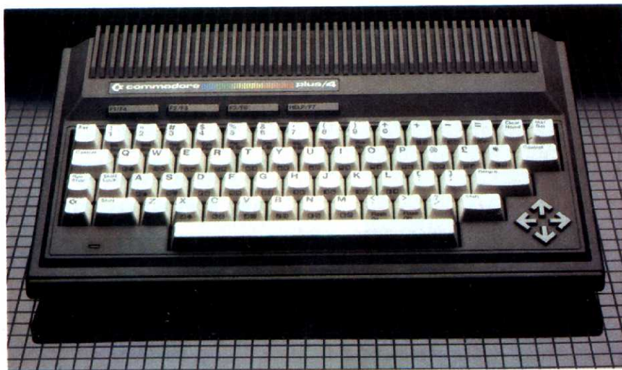
The Plus/4: unlike the C-64, the function keys are above the keyboard, the cursor keys are in a "compass configuration".
