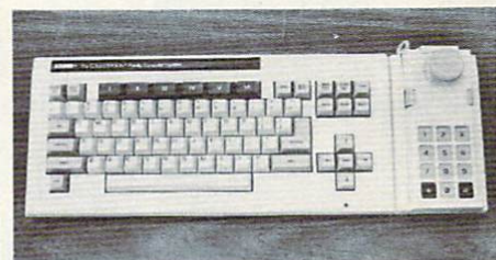
ADAM's keyboard is perhaps its strongest component. It has 75 keys plus a numeric keypad, and is easy to learn your way around and use.
