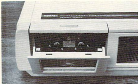
Coleco's digital tape drive, which runs programs stored on data packs, looks much like a cassette tape recorder. However, it is much faster, and can be operated under computer control. With data packs, which look much like cassettes, you can locate files or programs much faster than you can on cassettes.
