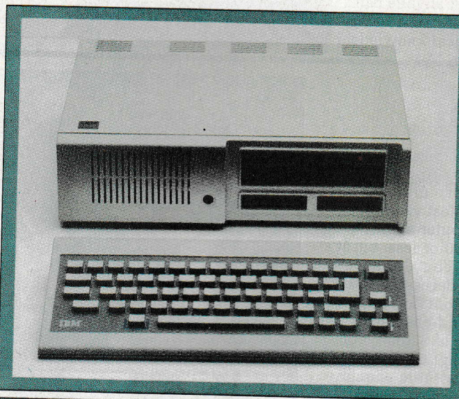
The IBM PCjr is the company's most affordable system. Based on the popular PC, the version shown features 128K of user memory, a double-density disk drive, two program cartridge slots and an infrared cordless keyboard. Cost is $1,269.
