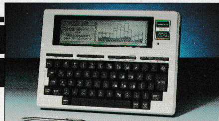
The TRS Model 100 has a full-sized keyboard, weighs less than 4 lbs. and comes with built-in software. It operates on 4 standard "AA" batteries.
