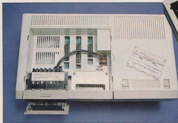
Above is the Adam's 80-column printer with its standard Diablo cartridge and daisywheels. At left is the main Adam processing box with cartridge software slot (bottom right), floppy cassette tape drive (bottom left) and plug-ins for further expansion (they are the slots pictured above the tape drive).
