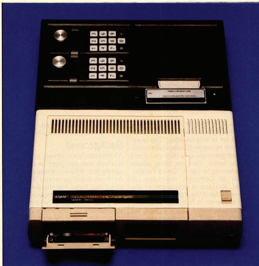
The memory module incorporates a 500k digital data-drive
