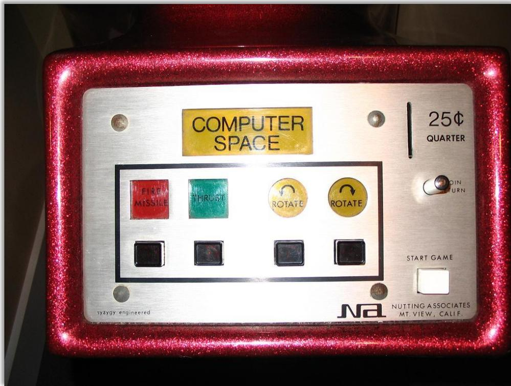
In fact, the first version of the control panel, seen in the game flyer, used a molded lever for directing the player's rocket ship, but Ted Dabney confessed many years later that kids kept breaking that controller off; hence the control panel was redesigned with push buttons for thrust, rotation and missile firing.
