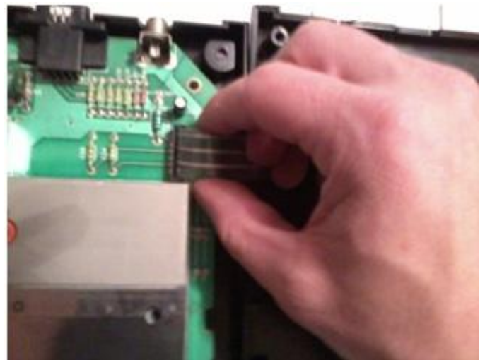
Removing PUSH Button Flex-Circuit from Main Board
