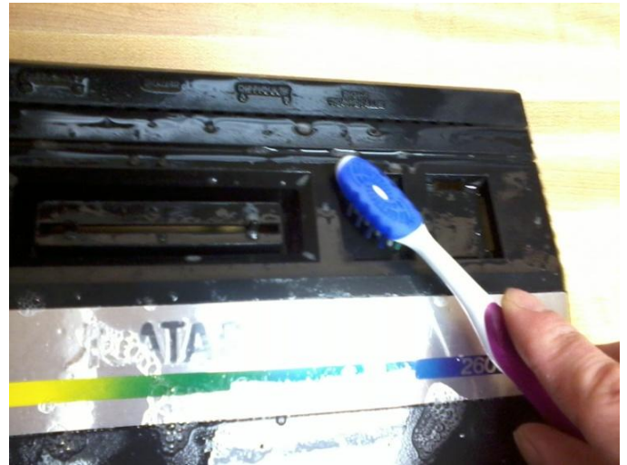
Using Toothbrush to Clean Button Recesses
