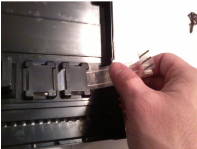
Removing Flex-Circuit Using Free End
